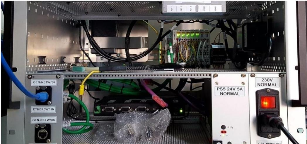
Figure 13: EtherCAT to RS-485 connection and NIR slit controller at INAF-OACN lab
